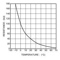
Fig.6 Thermistor curve
